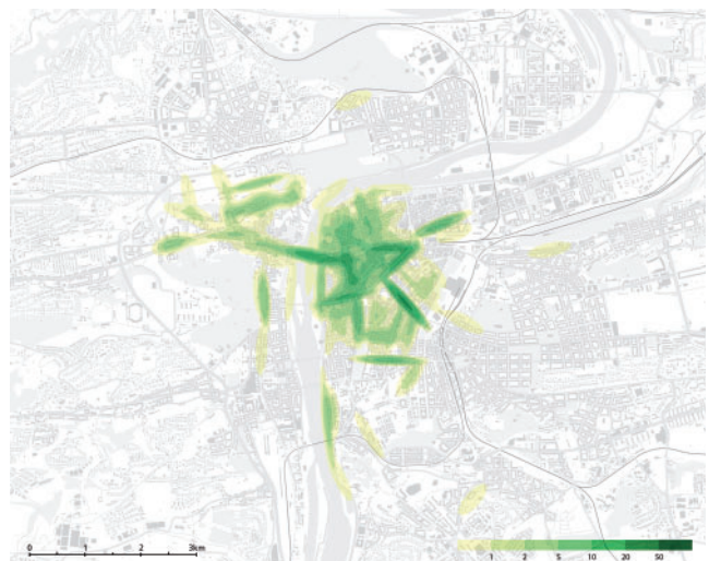
Figure 8. Density estimation for paths approximated by ellipses: a mean bandwidth of 50 pixels (315 m) and a minimal ellipse axes ratio of 1 : 5
